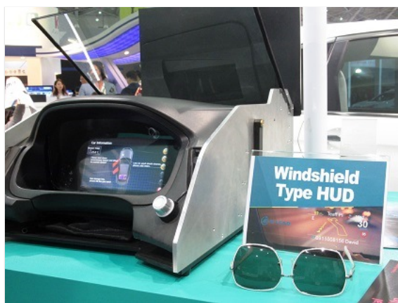
戴著墨鏡也能看清楚的擋風玻璃投影式HUD (來源：EE Times)
