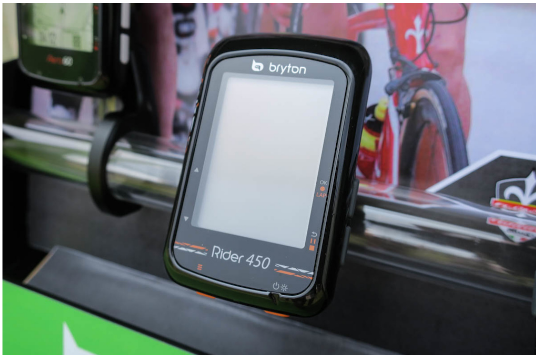
pb Bryton's upcoming $209 USD computer supports up to 72 functions, has Strava and TrainingPeaks auto sync, supports electronic shifting systems from Shimano, SRAM, and Campy, features smart notifications, and is ANT+/BLE compatible.
