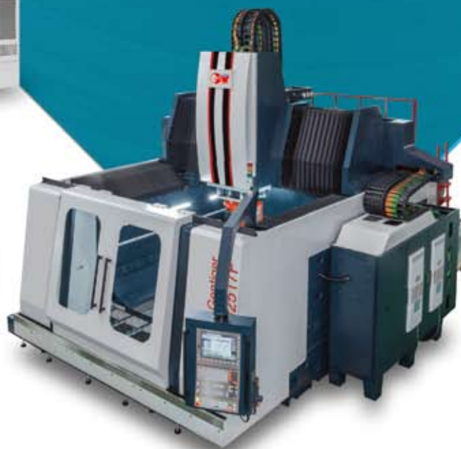
GT-H2517F Gantry type 5 axis High Speed Machining Center
