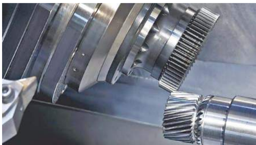
Efficiently geared by using the power skiving technology
