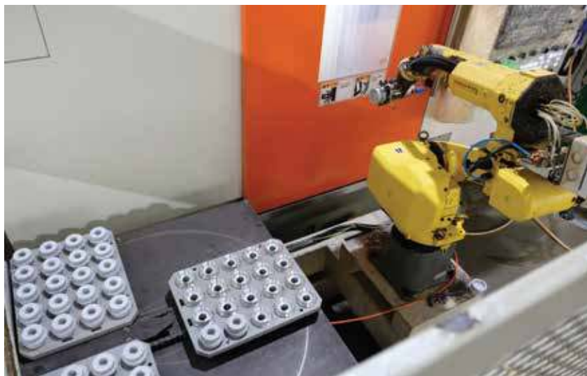
A robot feeds raw hub shells into a CNC lathe at Shutter Precision.
