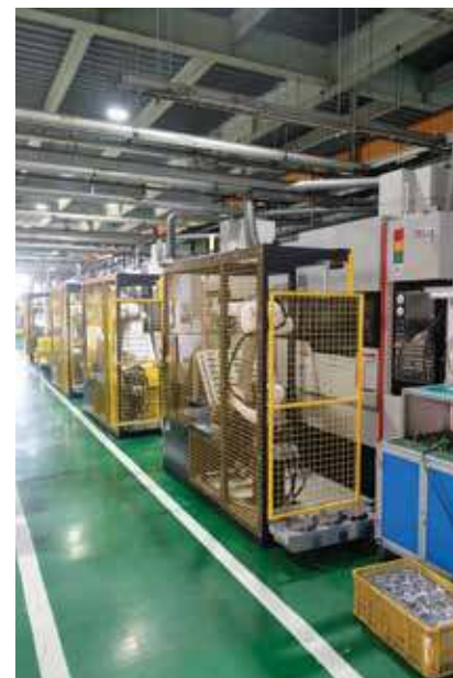
A line of CNC lathes fed by robots in Tektro-TRP's new factory hall.
