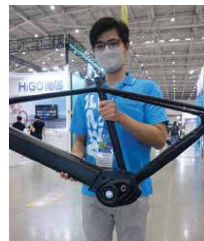
MPF offers neat frame brackets to make integration easy for frame makers
