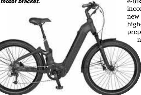
The new IQ8000 low step e-bike frame hides the shock right behind the seat tube for a clean design.
