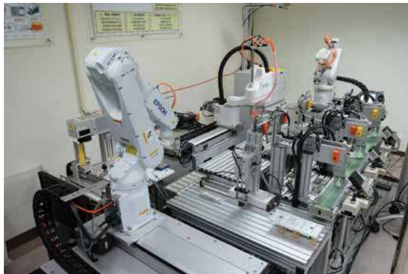
Robots from three different suppliers working together to assemble pedals as a test run.
