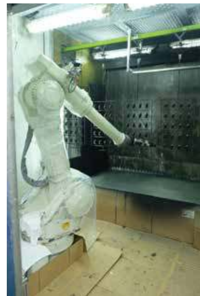
Tektro-TRP relies on robots in the paint shop as well.
