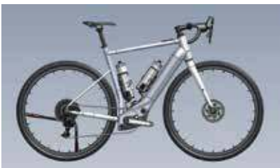
Kinesis' patented technology enables a single-piece hydroformed downtube and motor bracket.
